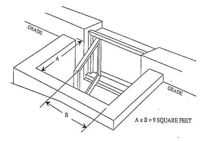
Window wells with a vertical depth greater than 44 inches below the adjacent ground level shall be equipped with a permanently affixed ladder or steps usable with the window in the fully opened position. The ladder or stairs shall be permitted to encroach a maximum of 6 inches.
