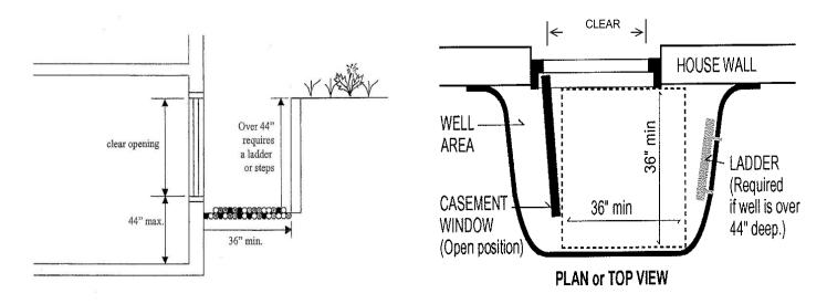
Window wells required for emergency escape and rescue shall have horizontal dimensions that allow the door or window of the emergency escape and rescue opening to be fully opened. The horizontal dimensions of the window well shall provide a minimum net clear area of 9 square feet with a minimum horizontal projection and width of 36 inches.
