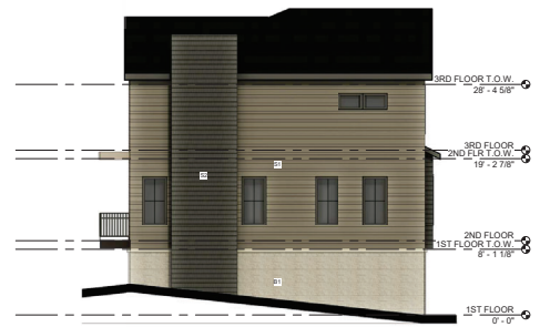
4 WEST ELEVATION - BUILDING 1 SCALE: 1/8" = 1'-0"
