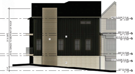
4 SOUTH ELEVATION - BUILDING 2 SCALE: 1/8" = 1'-0"
