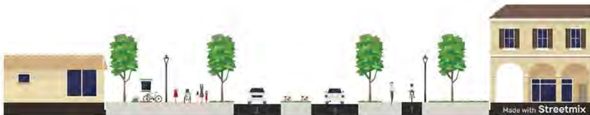
Complete street concept for County Road E – three lane cross section with center left-turn lane and medians between intersections east of Highway 61.
