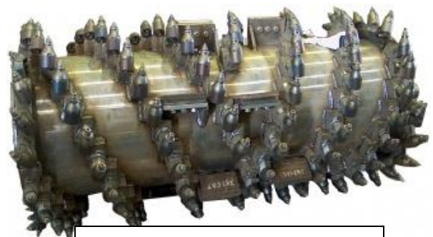
Grinding Drum from Milling Machine
