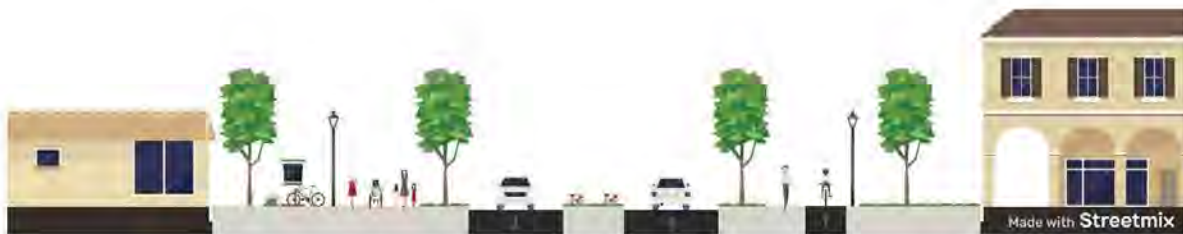
Complete street concept for County Road E – three lane cross section with center left-turn lane and medians between intersections east of Highway 61.
