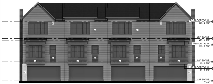
1 SOUTH ELEVATION - BUILDING 1 SCALE: 1/8" = 1'-0"
