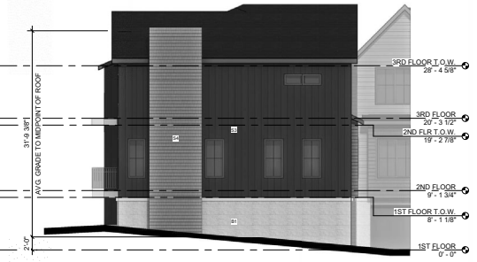
4 SOUTH ELEVATION - BUILDING 2 SCALE: 1/8" = 1'-0"
