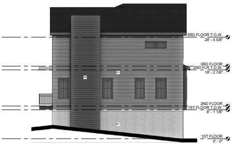
4 WEST ELEVATION - BUILDING 1 SCALE: 1/8" = 1'-0"
