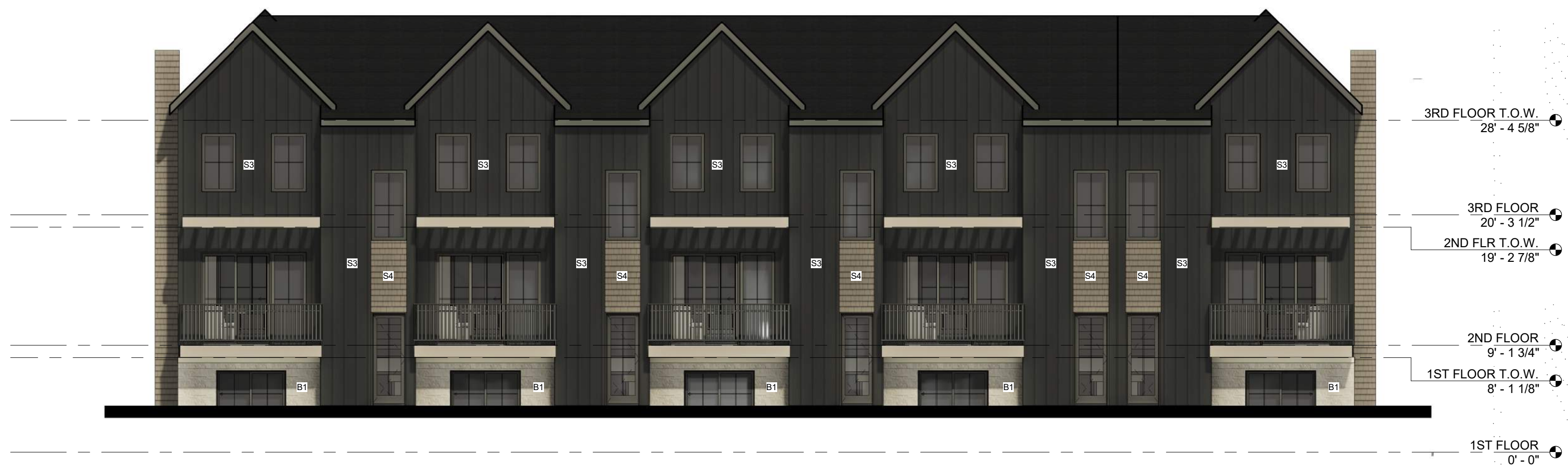
1 WEST ELEVATION - BUILDING 2 SCALE: 1/8" = 1'-0"
