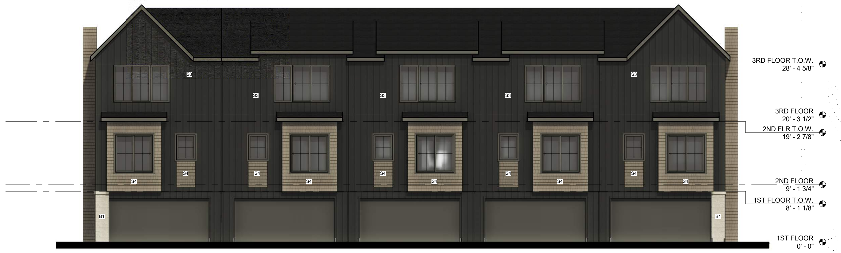
3 EAST ELEVATION - BUILDING 2 SCALE: 1/8" = 1'-0"
