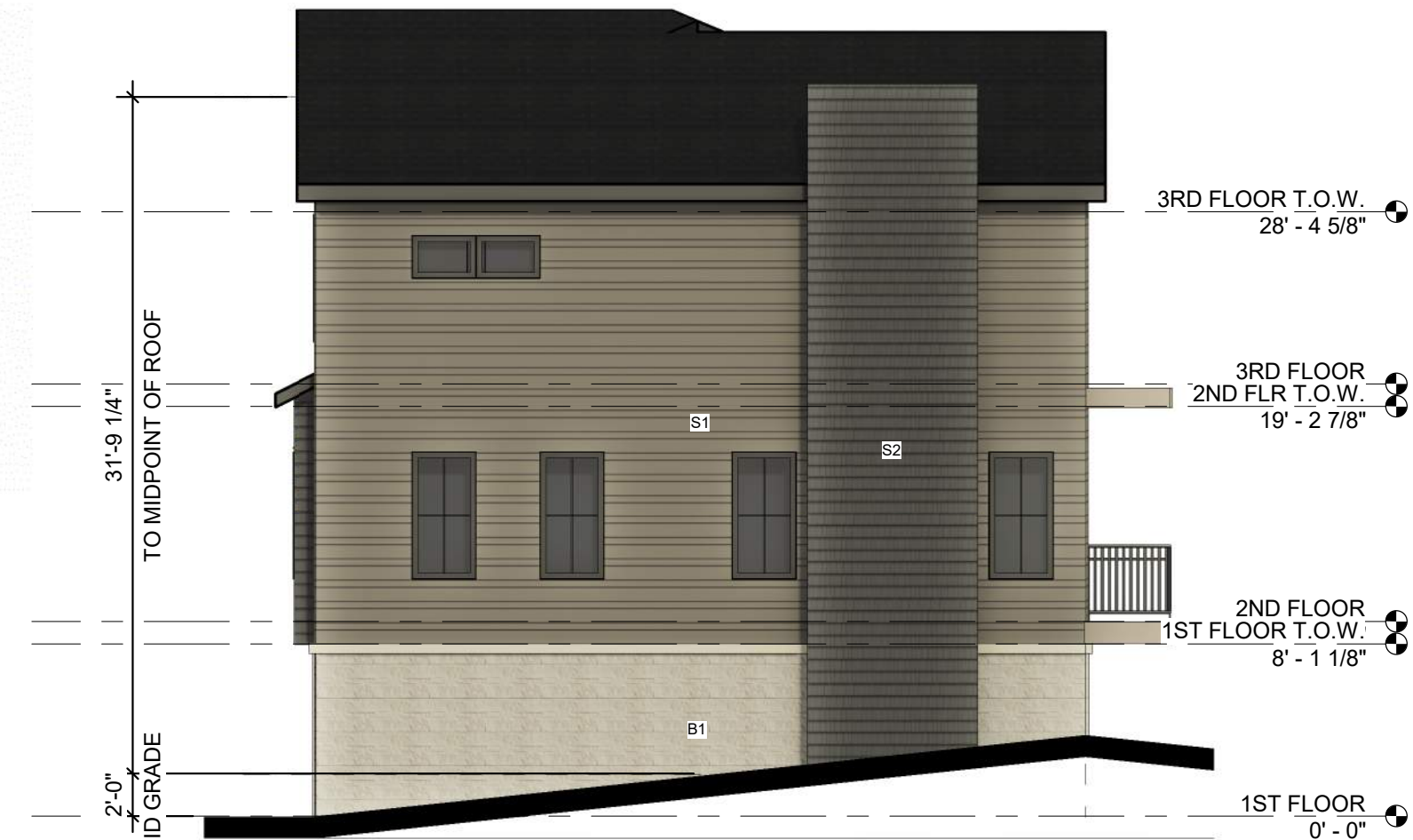
3 EAST ELEVATION - BUILDING 1 SCALE: 1/8" = 1'-0"
