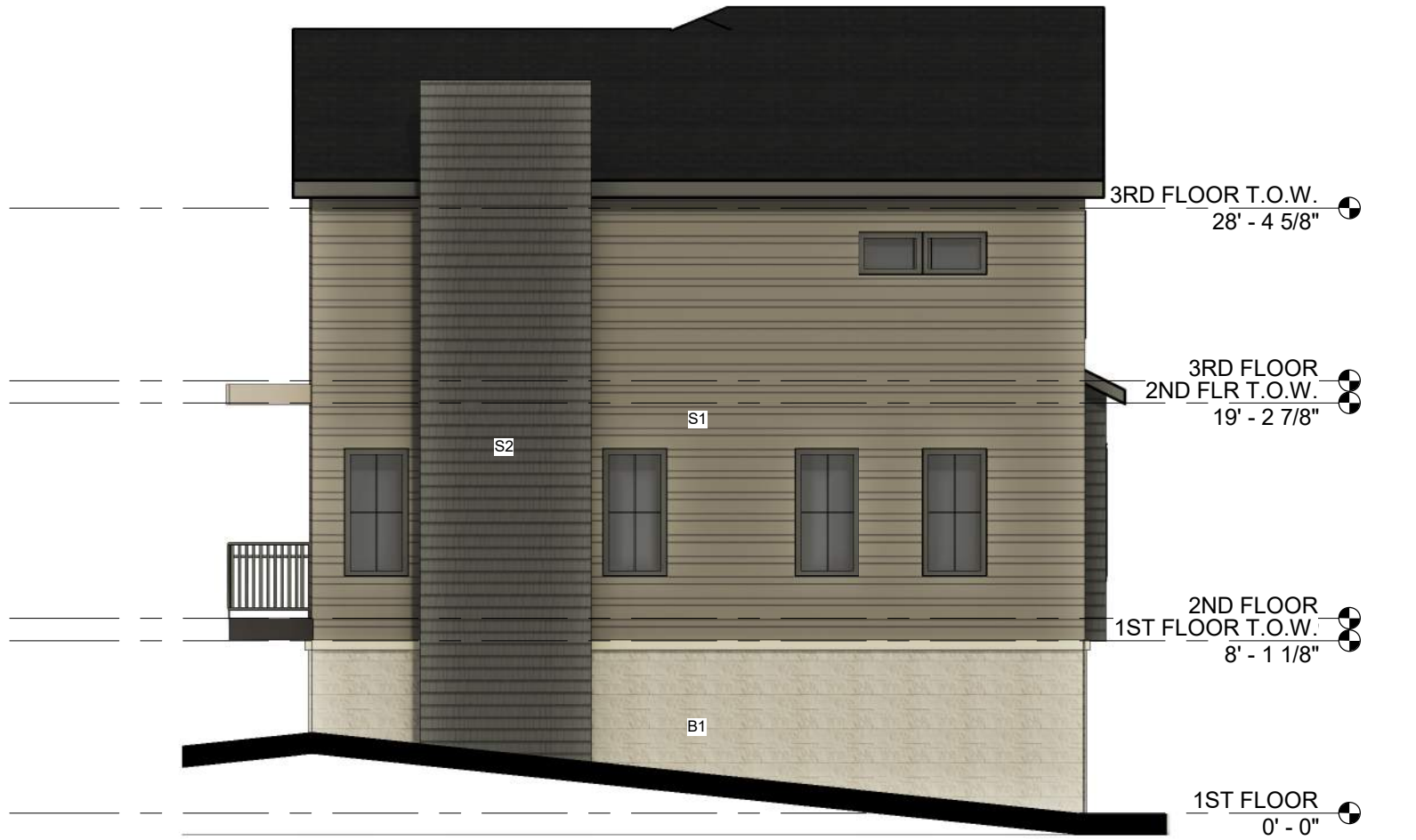
4 WEST ELEVATION - BUILDING 1 SCALE: 1/8" = 1'-0"
