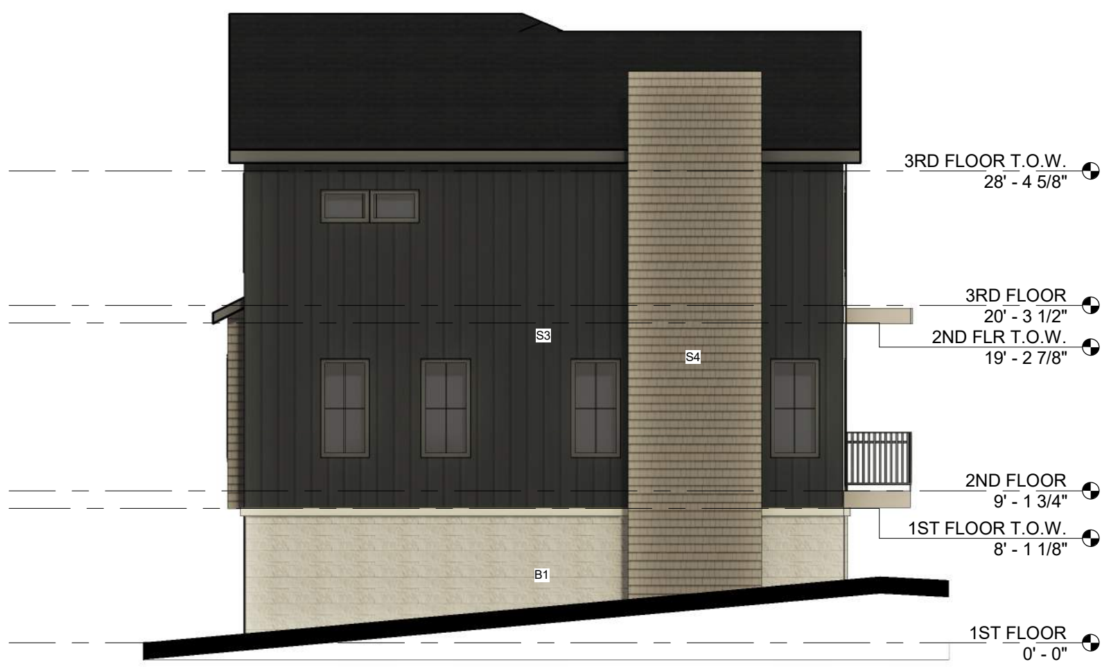
2 NORTH ELEVATION - BUILDING 2 SCALE: 1/8" = 1'-0"
