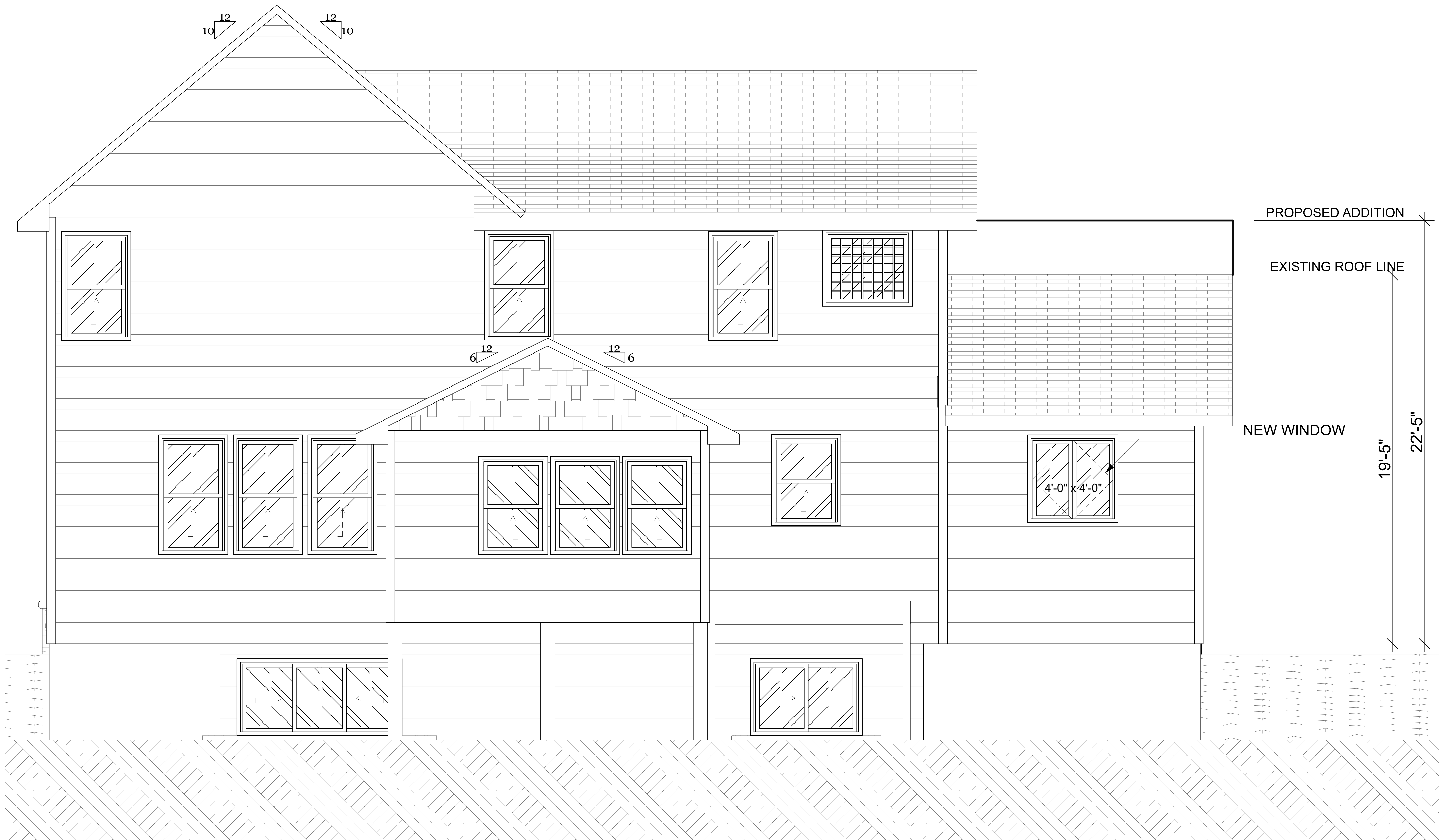
1 REAR/NORTH ELEVATION SCALE: 1:27,43
