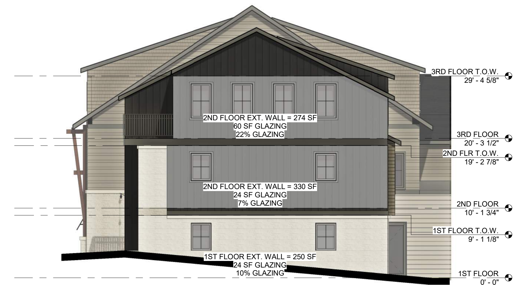
2 SOUTH ELEVATION - TOWNHOMES - GLAZING SCALE: 1/8" = 1'-0"
