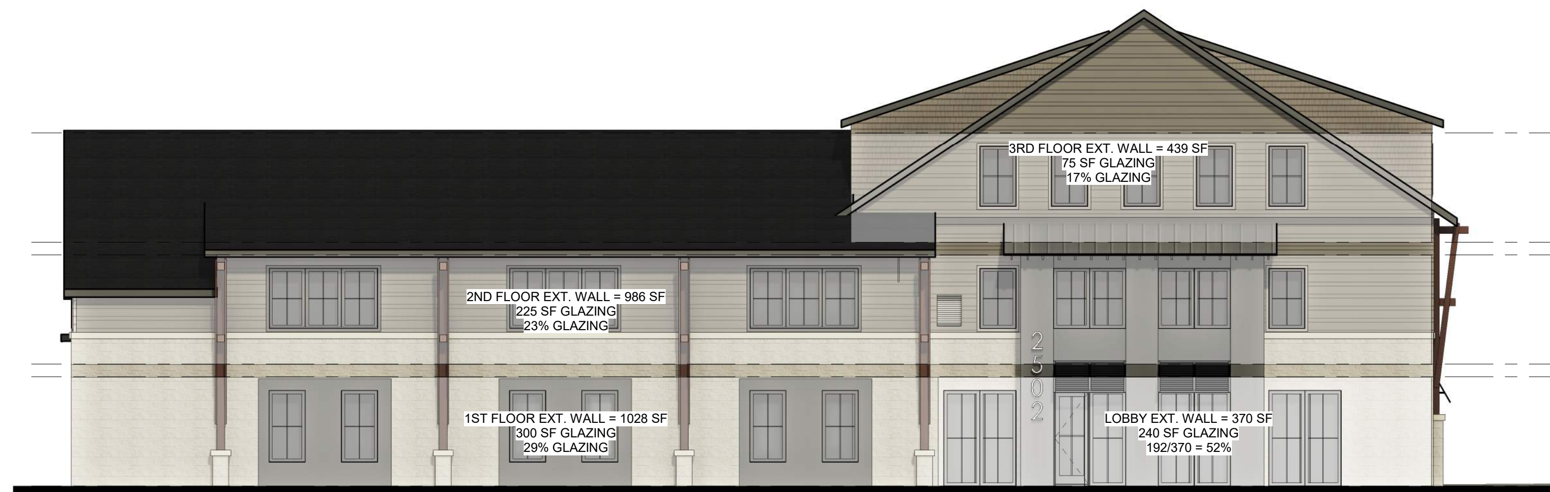
3 NORTH ELEVATION - GLAZING SCALE: 1/8" = 1'-0"
