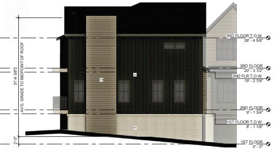
4 SOUTH ELEVATION - BUILDING 2 SCALE: 1/8" = 1'-0"
