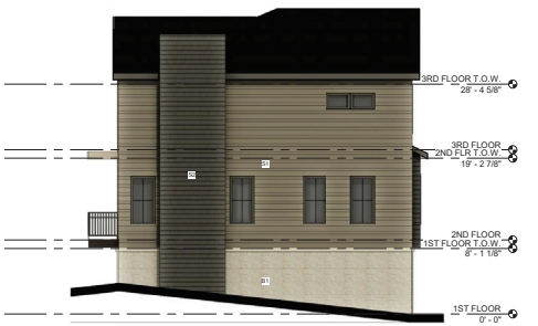
4 WEST ELEVATION - BUILDING 1 SCALE: 1/8" = 1'-0"
