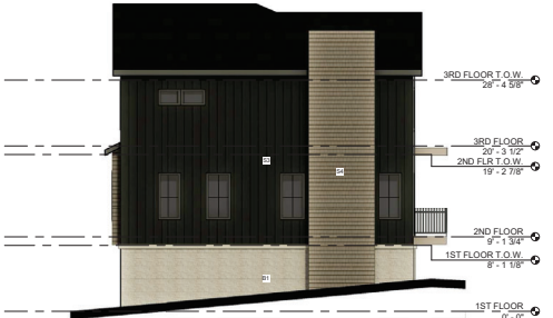
2 NORTH ELEVATION - BUILDING 2 SCALE: 1/8" = 1'-0"
