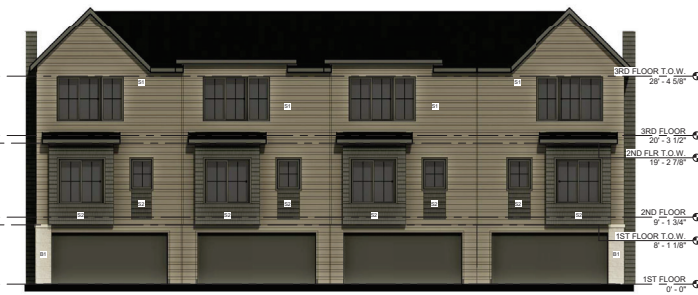
1 SOUTH ELEVATION - BUILDING 1 SCALE: 1/8" = 1'-0"
